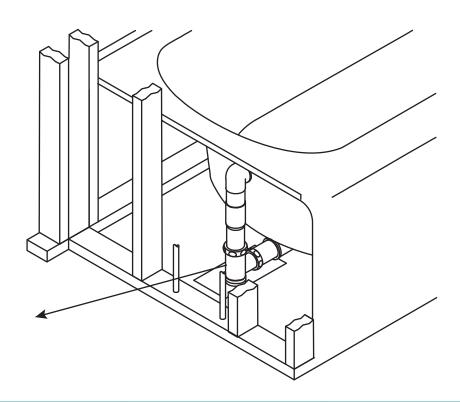
Connect the tub drain to your drain system.
