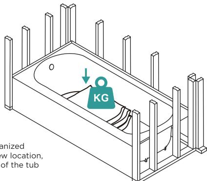
Secure to the wall with galvanized screws at the predrilled screw location, Apply weight to the middle of the tub until the mortar sets.
