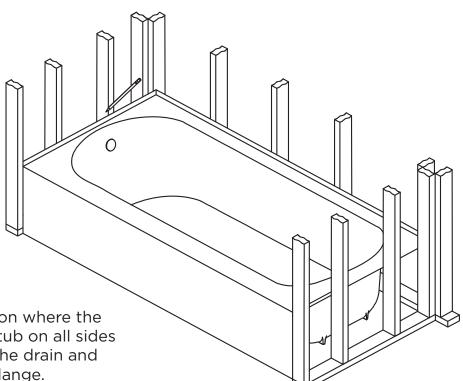
Place the tub at the location where the tub will be installed, level tub on all sides and mark the location of the drain and the wall studs on the tile flange.
